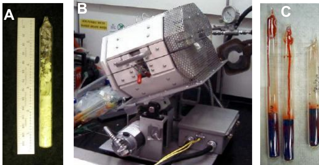
Figure 4.2: Synthesis steps for producing chalcogenide glass: (A) evacuated ampoules are made using high purity (=99.99%) elemental sources, (B) the ampoules are heated and rocked in a rocking furnace, and (C) the molten chalcogenide glass is quickly cooled to quench it into an amorphous state
